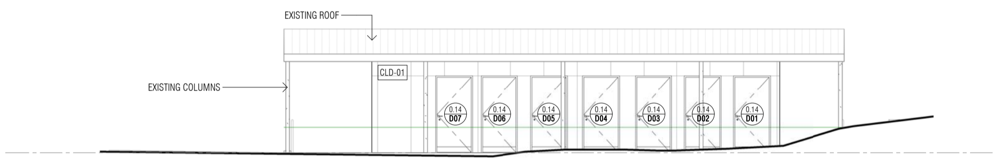
3 | PROPOSED TOILET BLOCK ELEVATION 1 1:100
